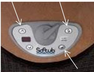
To enter this mode, Press and hold the **Light** button, **Jets** button & the **A** button together for 10 seconds, 12 will display on the control panel for 5 seconds to let you know that you have entered this mode. The heat and filter LED's will flash twice every 15 seconds to alert you that this mode is activated. The unit will not cycle on for twelve hours after entering this mode. The following 12 hours the unit will cycle when needed to filter/heat the water.
