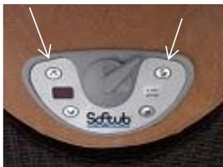
To enter this mode, Press and hold the **LIGHT** button and the **A** button together for 10 seconds, 24 will display on the control panel for 5 seconds to let you know that you have entered this mode. The filter LED light will flash once every 10 seconds to alert you that this mode is activated. When this mode is selected the unit will cycle once per day to filter/heat water. This cycle will occur at the same time each day this mode was activated.
